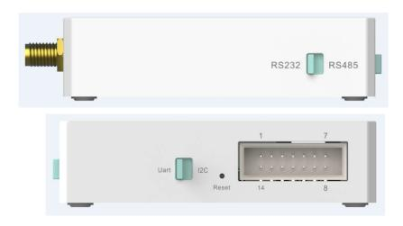
■ Interface: RS485, RS232, UART, I2C and GPIO (Output only)
